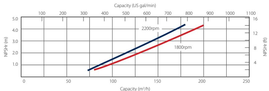
**Please note:** The above curve covers the complete range and ability of the pump unit. Actual performance will be subject to the motor/engine indicated overleaf.
